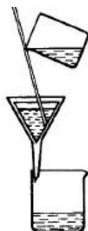
filtrace suspenze \text{Ca}(\text{OH})_2
